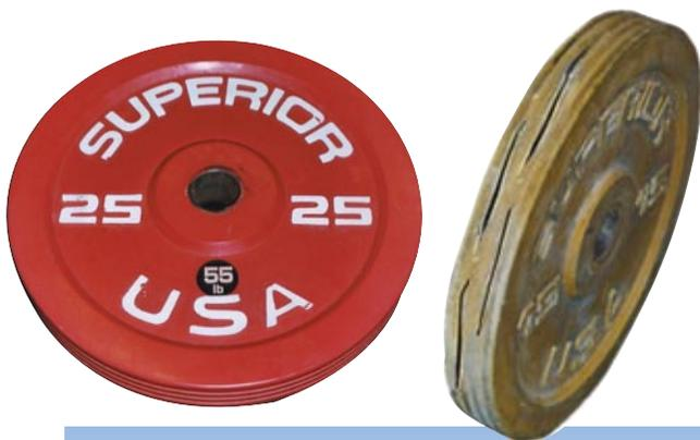
**The first Urethane Plates introduced in 1983 by Superior Barbell had problems with splitting. Like many other problems with rubber and urethane, this one was solved through a combination of reformulation and advances in urethane molding technology.**
