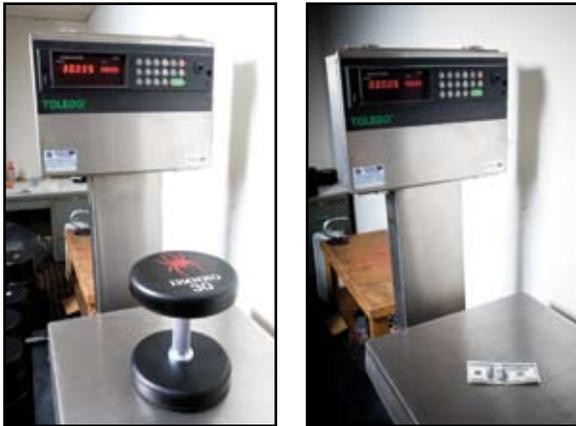
**Our specially made Toledo scale indicated this dumbbell accurate to 5-1000th of a pound, the weight of a \$100 bill.**
