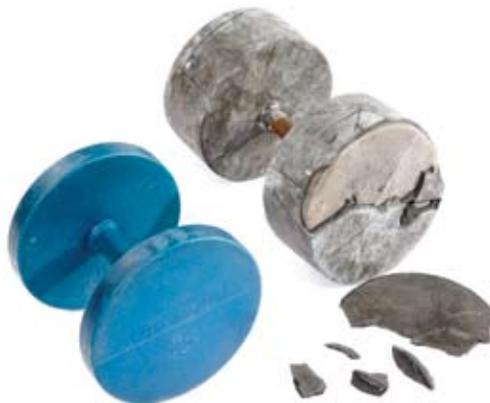
**The first urethane dumbbells by Universal in the 1980's developed cracking and peeling over time. Time will tell whether other brands will develop similar problems.**
