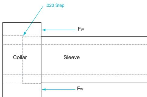
The addition of a .020" step increases the interface pressure from 63,000 psi to 139,000 psi for the interference fit compared to 51,000 psi for welding at both ends.
