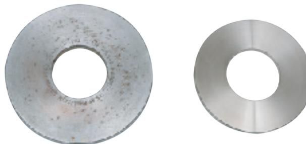
**After Cleaning:** The cleaned and polished chrome plate on the left exhibits residual pitting and discoloration, while the stainless steel plate on the right cleaned up “good as new”.
