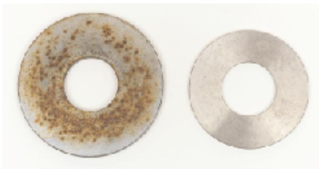
**Before Cleaning:** After two years of “Roof Test” exposure, the chrome plate on the left exhibits considerable rust while the stainless steel plate on the right is only slightly blemished.
